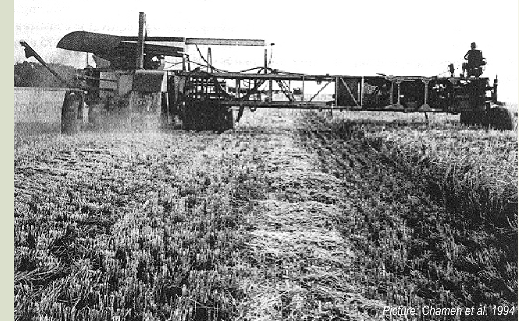
12-m gantry with combine harvester
