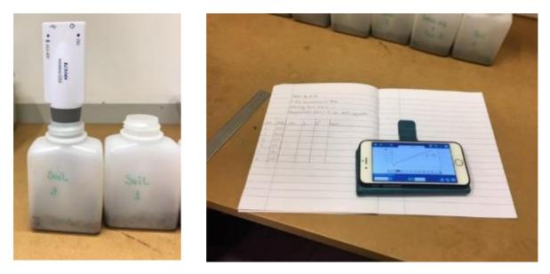
**Photo 8.** Left side: Pasco wireless CO<sub>2</sub> sensor during measuring the increase in CO<sub>2</sub> concentration inside a bottle with soil. Right side: Real-time measurement displayed on the mobile screen. Photos: Reidun Pommeresche, NORSØK.
