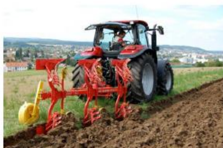
The on-land plough helps prevent soil compaction in the plough pan.
