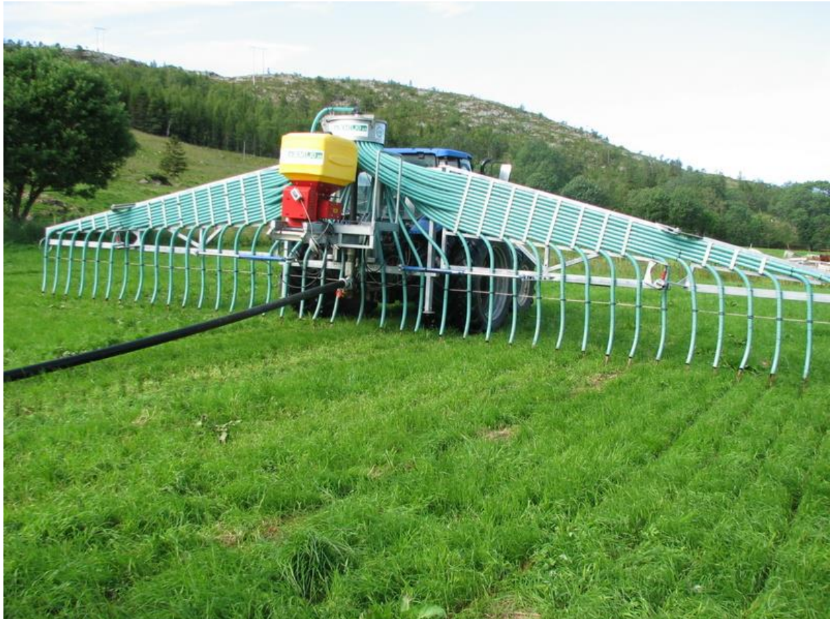
Figure 11: Drag hose with dribble bars for manure spraying.
