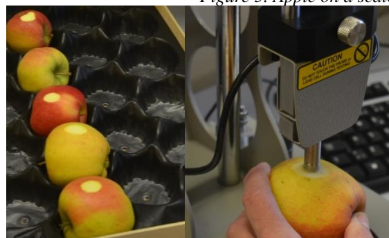
Figure 6. Five apples lined up and prepared for measurement of firmness (left) and analysis in progress (right).
