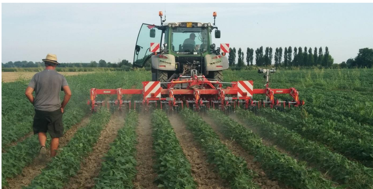
Picture 1: Hoe operating on soybean with camera assistance. Date: 23-07-2015 (Cristina Micheloni)
