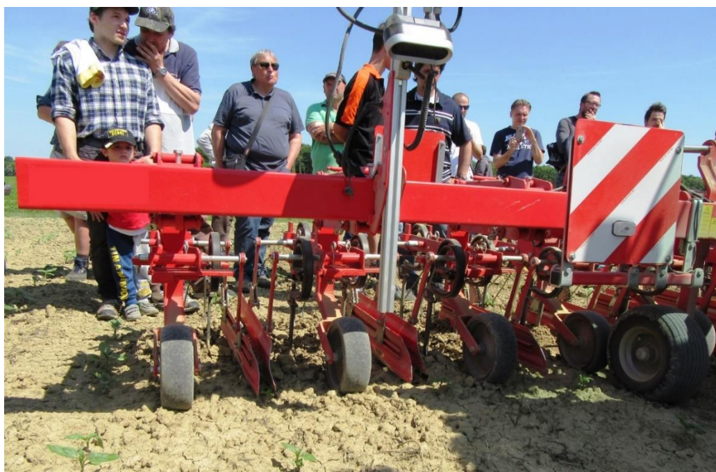
Picture 2: Hoe operating on sunflower with camera assistance. Date: 21-05-2016 (Gemini Delle Vedove)
