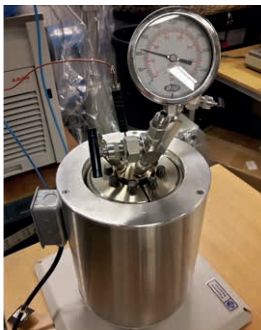
Parr reactor (250 ml) for hydrothermal carbonization. Photo by Judit Sandquist, SINTEF Energy Research.
