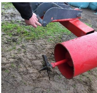
Picture 1: The dock-cutter is mounted on a mini-loader. Picture 2: The drill/cutter of the dock-cutter. Picture 3: The WUZI dock-cutter in action drilling out a dock. (Photos: Casper Laursen, SEGES).
