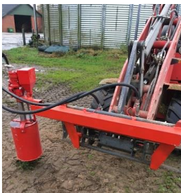
Picture 1: The dock-cutter is mounted on a mini-loader. Picture 2: The drill/cutter of the dock-cutter. Picture 3: The WUZI dock-cutter in action drilling out a dock. (Photos: Casper Laursen, SEGES).
