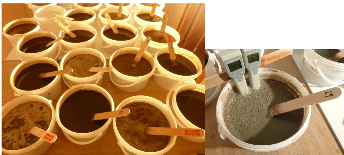
Picture 1: Open containers filled with pig slurry, Ecopro digestate, cow slurry or digested cow slurry (left), to measure pH and red-ox potential over time (right) and to measure losses of N during six weeks with repeated stirring. Photos by Reidun Pommeresche.
