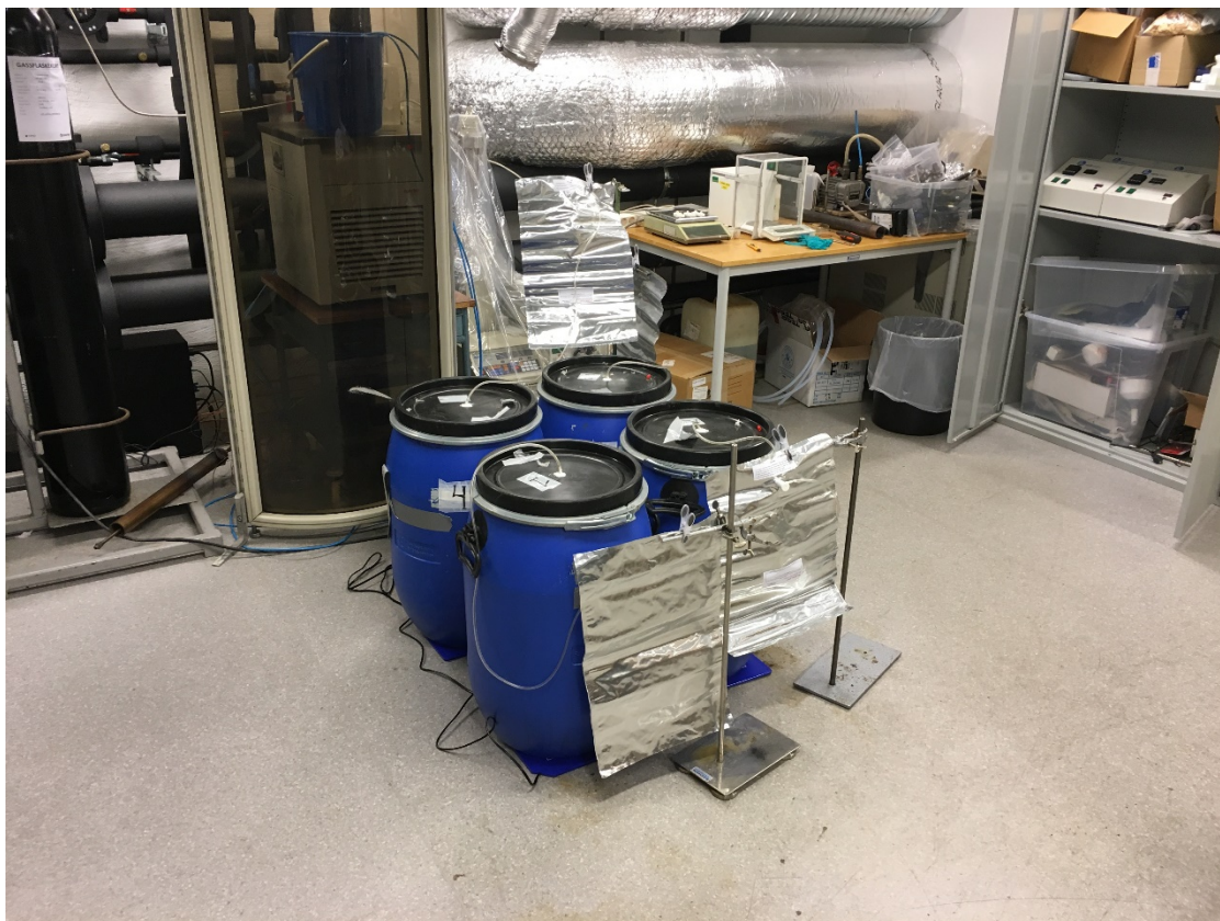
Picture 2. Containers with Ecopro digestate ready for collection of gas at SINTEF Energy Research, Trondheim. Photo by Roger Khalil.
