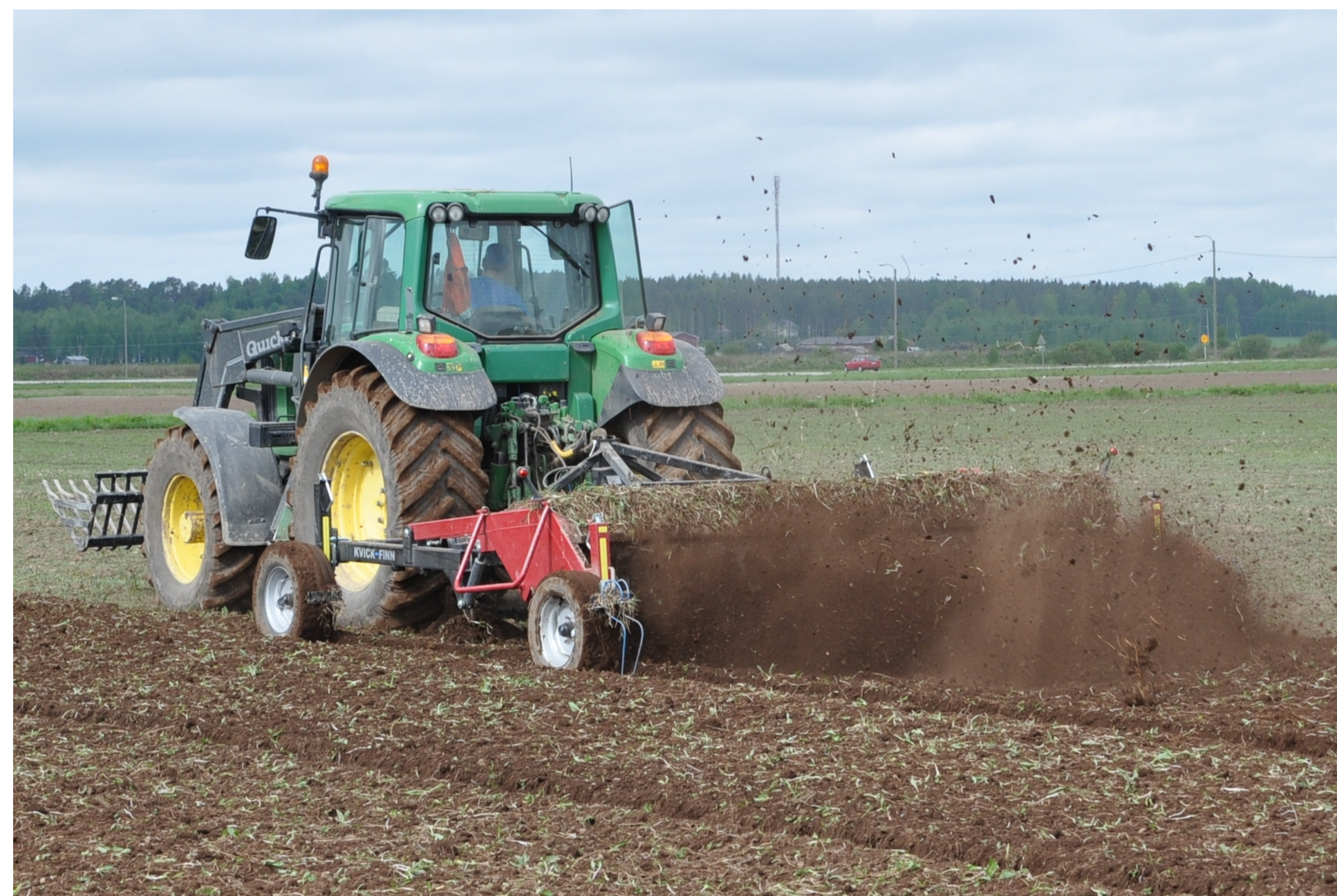
Figure 1. Kwick-Finn cultivator lifts the roots or rhizomes of perennial weeds to the soil surface so that sun and wind can desiccate them. Goosefoot tines loosen the soil and after that a PTO-driven rotor throws soil and weed roots into the air.
