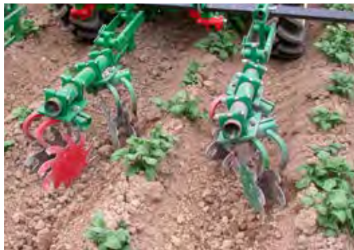
The rotary hoe is well suited for earthing up the ridges on heavy soils.
