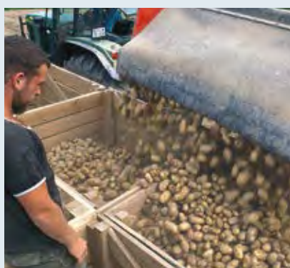
Fall heights above 25cm should be avoided to prevent impact damage.
