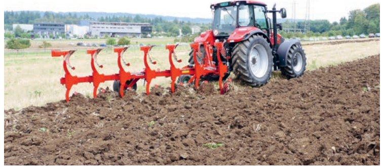
The skim plough (picture: a Ovlac skim plough) allows precise superficial tillage due to the support wheel.
