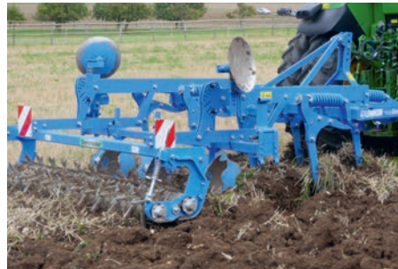
The skim plough (picture: a Ovlac skim plough) allows precise superficial tillage due to the support wheel.
