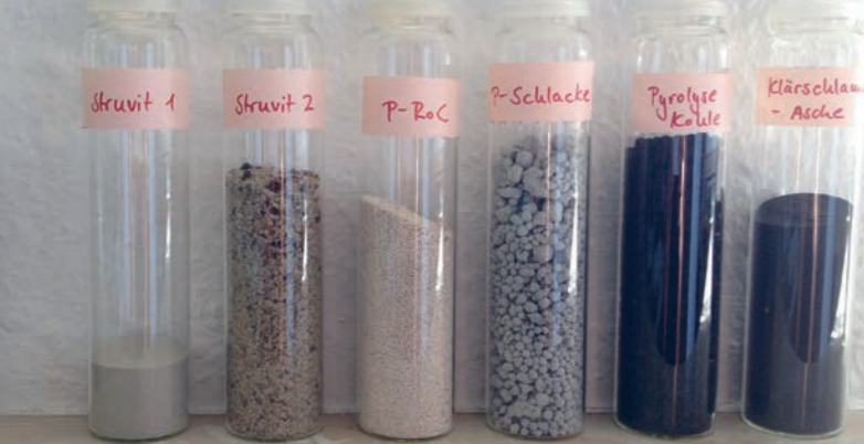
Recycled phosphorus fertilizers based on sewage sludge: from left: two struvites, Ca-phosphate, converter slag, biochar, biosolids ash.
