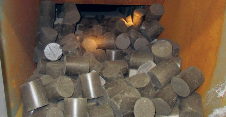
Dried sludge pressed into briquettes before thermal treatment in a shaft furnace of a Mephrec-test facility at temperatures above 1,450°C.
