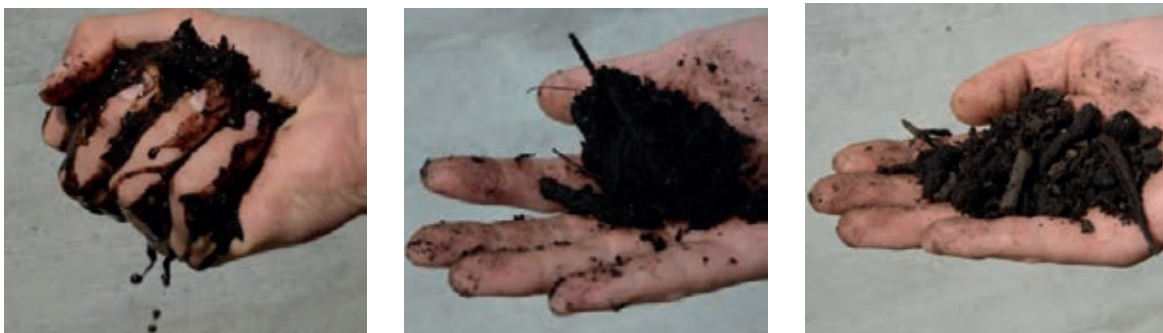
Figure 4.5 Fist test to control the humidity of compost during the composting process. From left to right: too wet, optimal, and too dry.
