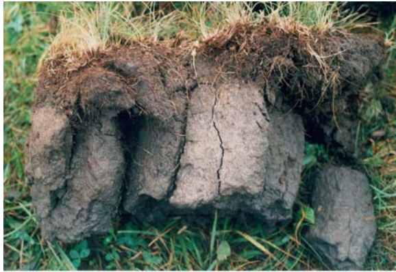
Fig. 3.3.3.-1: Coarse columnar structure of a Solonetz. Grassland vegetation is adapted to low to moderate sodification, score 1.5, multiplier 2.8. Location at Neusiedler See, Austria (Nelhiebel et al., 2001).
