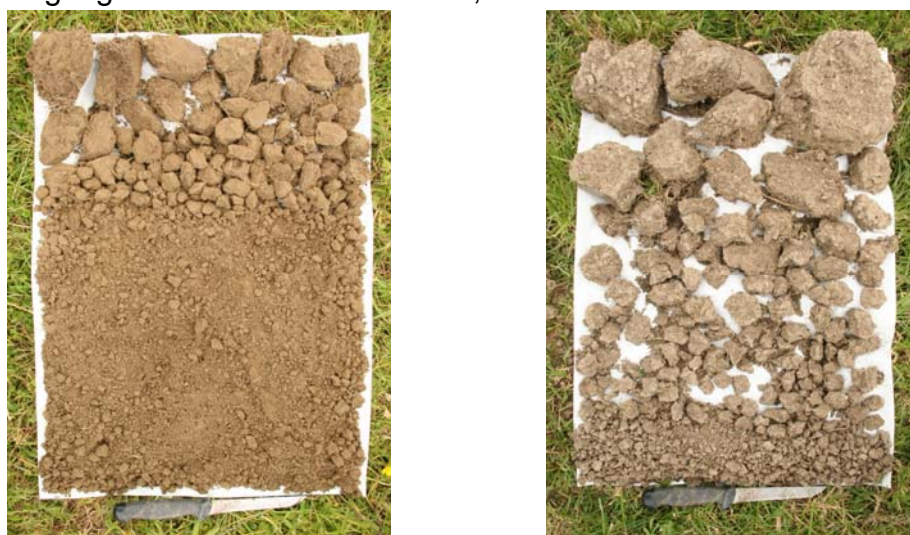
Fig. 3.2.3.-1: The arrangement of aggregates after performing the drop-shatter test of the VSA procedure (Shepherd, 2000) indicates differences of soil structure. The Manawatu soil (NZ: Weathered Fluvisol recent soil, FAO WRB: Eutric Fluvisol) shows moderate to good structure conditions (score 1.5) whilst the very clayey Kairanga soil (NZ: Typic Orthic Gley, FAO WRB: Eutric Gleysol) has a high proportion of large blocky aggregates (score 0). Performance of the VSA procedure is recommended in conjunction with the Muencheberg SQR.
