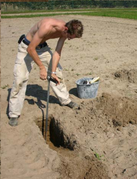
Fig 3.1.-4: From the bottom of the soilpit a hole will be bored to detect soil layering and a shallow watertable.
