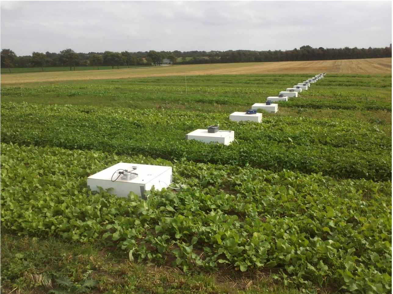
Photo 1, chambers for N 2 O measurement in the field, 10/09/2012.
