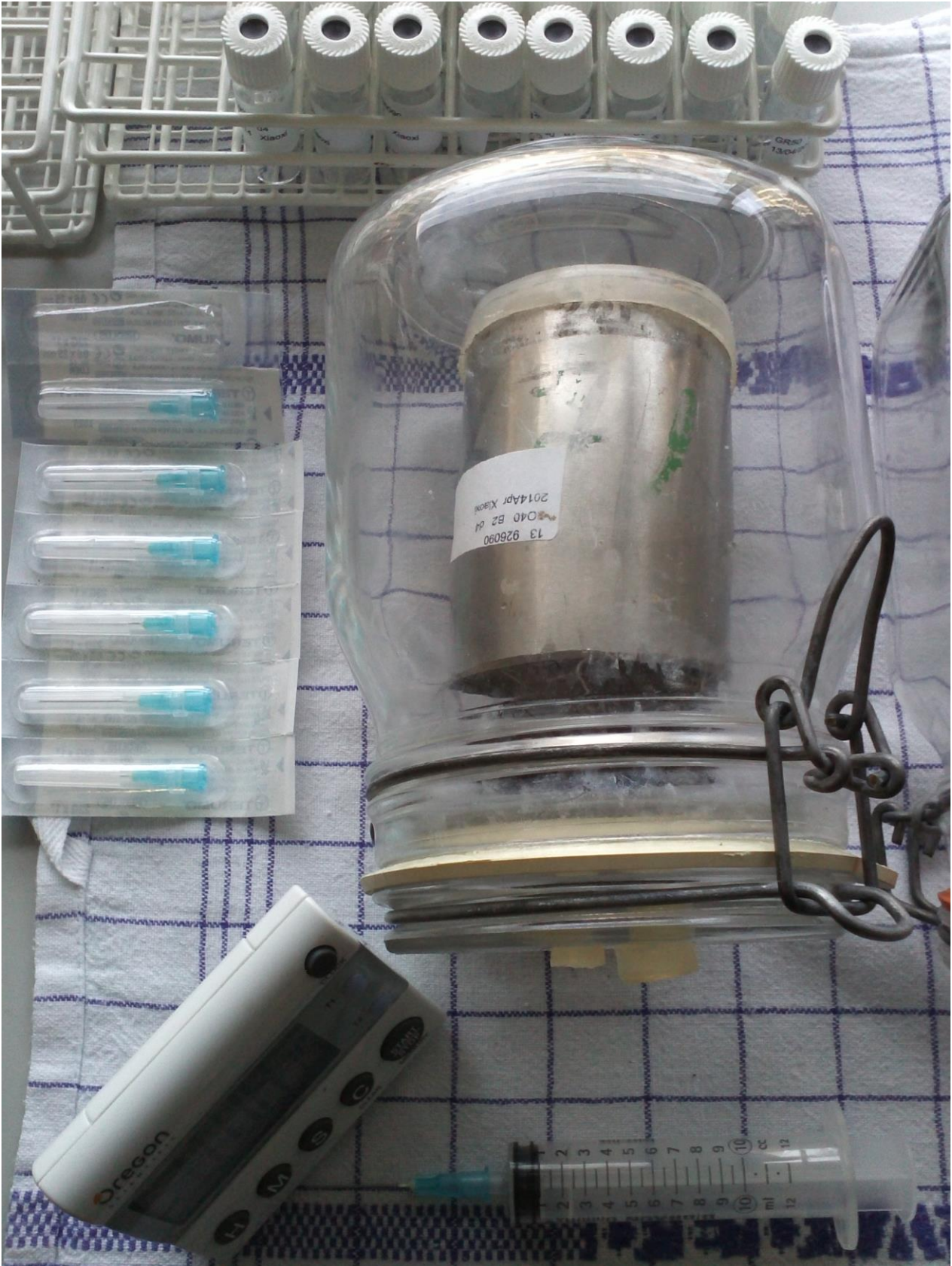
Photo 4, an incubation soil core with catch crop residue addition in a glass jar ready for N 2 O measurement, 13/04/2014 (lab study).
