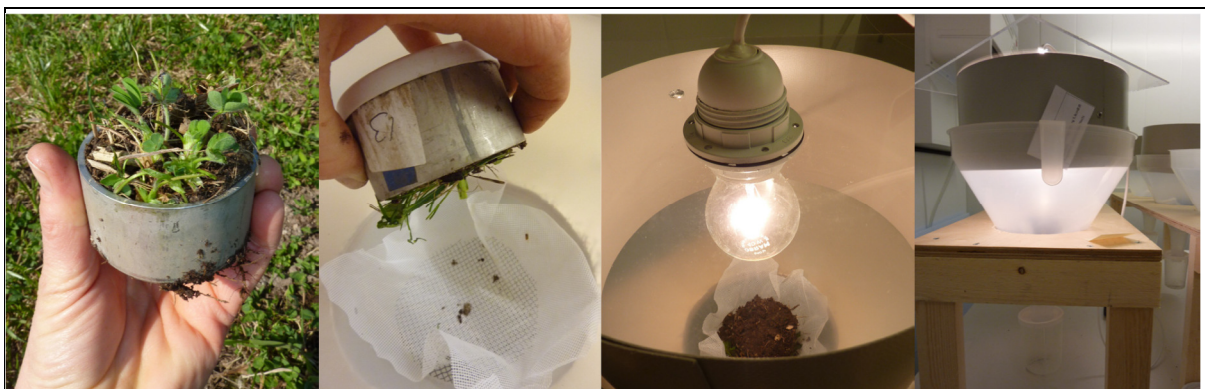
Figure 7.8. Sampling and extraction of collembolans. From left: Soil and sward is sampled by means of a metal cylinder that is tapped into the ground and excavated. The sample is carefully placed, upside down, on a nylon net which allows collembolans to pass through, and placed under a lamp which forces the animals to redraw through the soil and further through the net. Animals are caught via a funnel in a bottle below the lamp. The bottle contains 80 % ethanol to conserve the animals.
