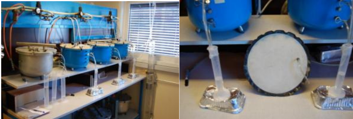
Figure 4.5. Equipment used for moisture retention analysis. Left: Pressure chambers, valves and manometers (Soil Moisture Inc.) Right: Ceramic suction plate for samples (3 plates per chamber).
