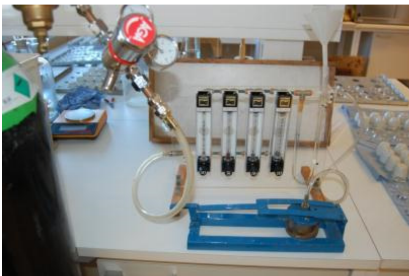
Figure 4.6. Flow-meter (Platon) setup used for measuring air permeability in soil cores at field capacity (Kise Res. Stn.).
