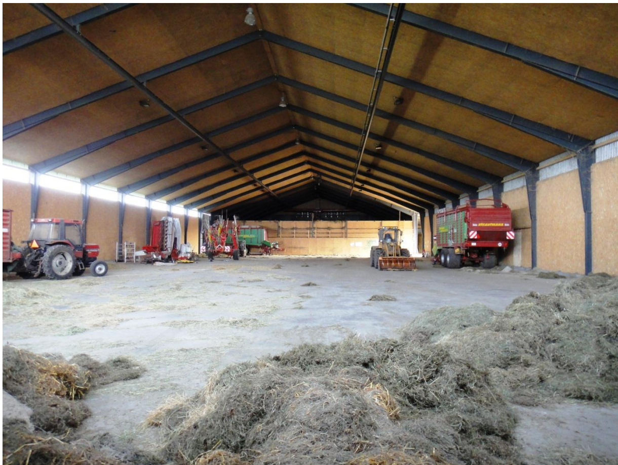
Figure 4.1: Barn for storage and drying of hay. Drying boxes are at the end Photo: Jesper Lehmann
