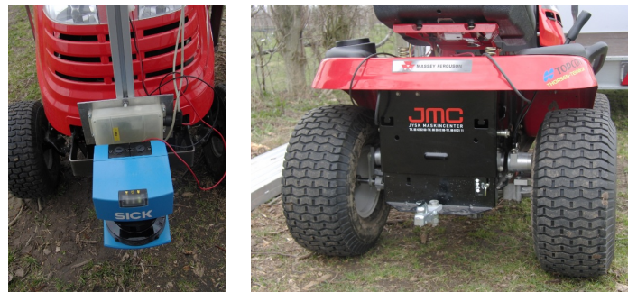
Figure 2: Placement of the IMU, LIDAR and Encoders on the tractor
