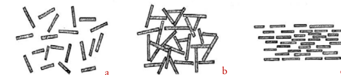
Figure 1. Clay particles dispersed in water (a), edge-to-edge flocculated in interaction with organic matter (b) or face-to-face cemented in lack of organic matter (c).
