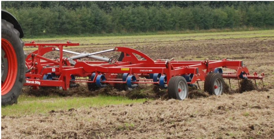
Fig 3: The spring loaded S-tine cultivator. A close up of the shape of the S-tines are displayed to the right (MARSK STIG Model 8).
