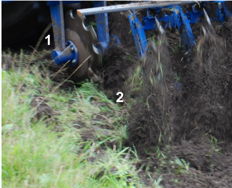
Fig 2: Spike disc cultivation. 1) row of standard concave discs, 2) row of spike discs.
