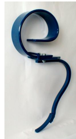
Fig 3: The spring loaded S-tine cultivator. A close up of the shape of the S-tines are displayed to the right (MARSK STIG Model 8).
