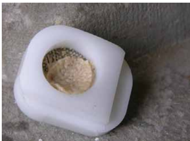
Figure 2 6 Determination of Gluten Index (GI): Gluten after centrifugation. Centrifugation allows for determining the amount of weak and strong gluten. Amount of weak gluten of a wheat cultivar with a high portion of weak gluten resulting in low GI. Source: Getreidezüchtung Peter Kunz
