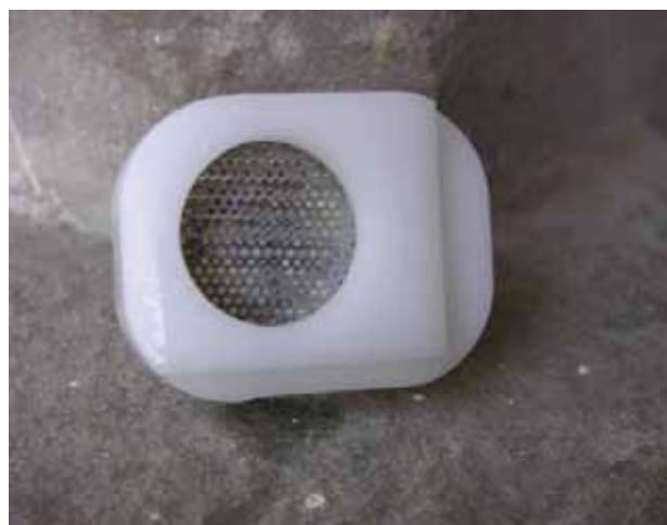
Figure 2 7 Determination of Gluten Index (GI): Gluten after centrifugation. Amount of weak gluten of a wheat cultivar with a high portion of strong gluten resulting in high GI. Source: Getreidezüchtung Peter Kunz
