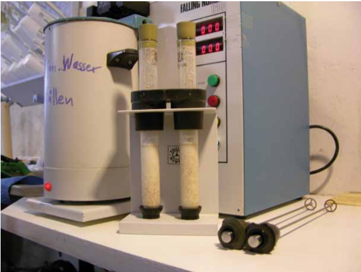
Figure 2 1 Determination of the falling number: Whole wheat flour with water with a stirrer inserted, is boiled in hot water. After 5 seconds the stirring begins automatically. The stirrer is automatically released in its top position after 60 seconds and is allowed to fall down under its own weight. The total time in seconds from the start of the instrument until the stirrer has fallen a measured distance is registered as the falling number. The flour is undergoing liquefaction due to alpha-amylase activity. The higher the alpha-amylase activity, the faster the liquefaction starts and the lower is the falling number. Rainy weather during harvest can cause sprouting leading to a development of the alpha-amylase enzymes. Alpha-amylase activity has direct impact on bread making quality. As little as 5 % sprouted grain, mixed with 95 % sound grain, can render the entire mixture unacceptable. Source: Getreidezüchtung Peter Kunz
