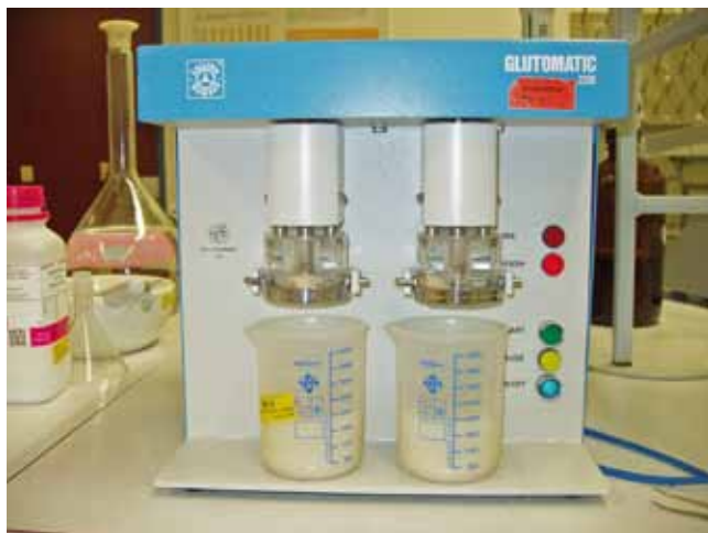
Figure 2 4 Determination of total wet gluten: Preparation of dough from whole meal flour by adding a sodium chloride solution. Total wet gluten is isolated by washing this dough with the same solution removing the residual water by centrifugation and weighing the remainder. Source: Isabell Hildermann
