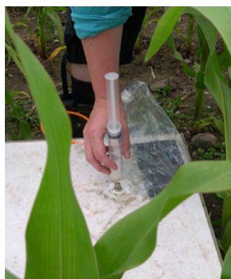
Figure 2. Emission of N 2 O was measured by manual gas sampling in gas-flux chambers.
