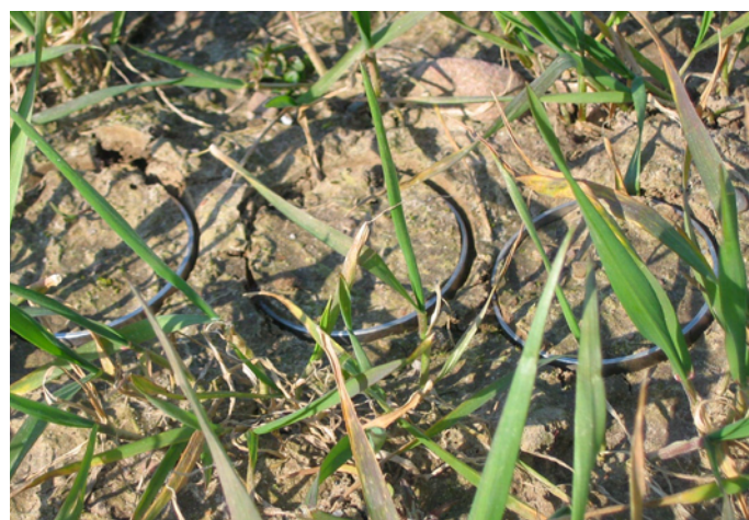
Figure 1a. A total of 72 100-cm 3 rings were installed at each site in November, shortly after seeding of winter wheat. They were randomly sampled in April, May, June and August the following year. Photo: Søren O. Petersen.
